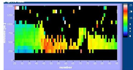
FIGURE 2: A lidar quick-look of the Hinlopen jet. The wind blows from left to right, and the maximum wind is at the mouth of the strait.
