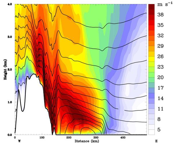
FIGURE 6: Simulated wind speed and isentropes (every 2K) in the cross section indicated in Fig.5.
