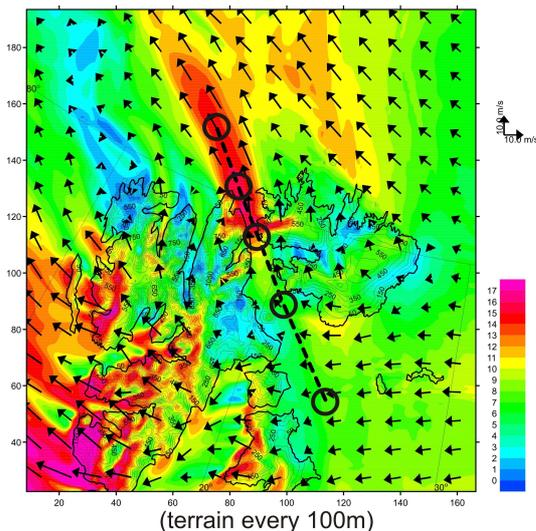
FIGURE 1: Wind speed at 210m height as indicated by the colorbar to the right. Circles indicate dropsondes positions. Terrain contours every 100m starting at 50m elevation are shown.
