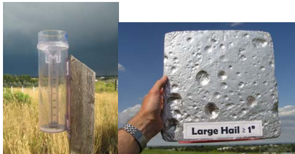
Figure 1. CoCoRaHS Rain Gauge and Hail Pad
