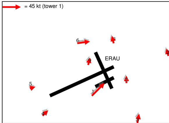
Fig. 12. LLWAS-derived wind analysis for 18:37:47 UTC. Vectors shown in red, with length proportional to speed. The DAB runway complex is shown schematically, and the location of the western edge of the ERAU campus, which is where the tornado touched down, is indicated by the letters “ERAU”.
