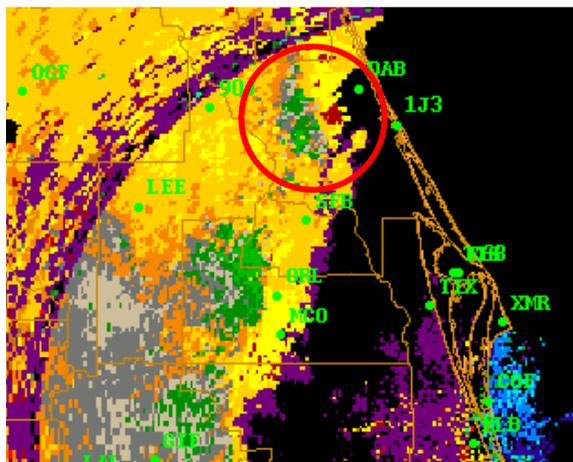
Fig. 10. WSR-88D storm-relative velocity scan for 1824 UTC. Light green shading within red circle indicates inward storm-relative velocities around 15kt, while the maroon shading nearly adjacent to it indicates outbound storm-relative velocities around 30kt, indicating a broad area of rotation as the storm approached the airport (indicated by 'DAB' with green dot denoting location).
