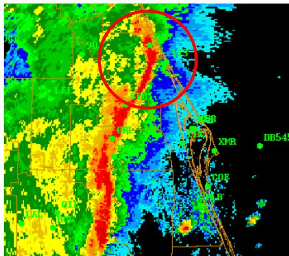
Fig. 11. WSR-88D composite reflectivity scan for 1837 UTC. Highest reflectivity values are 55dBZ, shown by maroon shading. Location of bowing echo segment is shown by red circle. Location of Daytona Beach International Airport (DAB) denoted by green dot. The squall line is passing through DAB at the time of this scan. The National Weather Service Forecast Office in Melbourne, Florida, determined tornado touchdown at DAB to be 1345 EST (1845 UTC).
