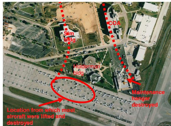
Fig. 14. Overhead photo of ERAU parking ramp and west side of campus, taken about a day after the event. Annotations of damage and estimated path were added by the author (photo courtesy of S. Keating).
