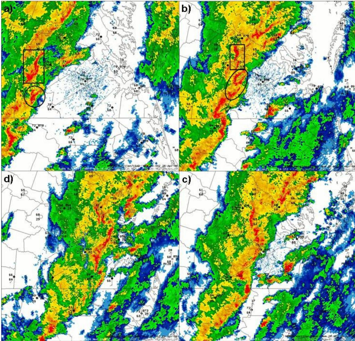
Figure 6. AKQ 0.5° reflectivity showing the QLCS and leading supercells as they progressed through the AKQ CWA at: a) 1855 UTC, b) 1937 UTC, c) 2006 UTC, and d) 2045 UTC with hourly surface METAR observations.
