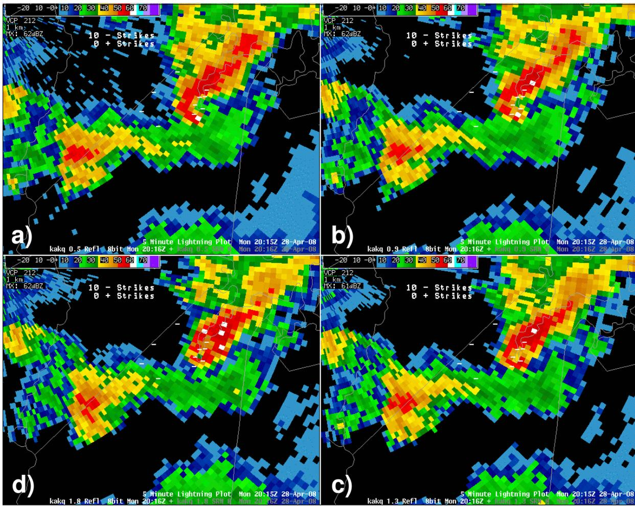
Figure 9. Same projection as Fig. 8, with 2016 UTC reflectivity over the city of Suffolk at: a) 0.5°, b) 0.9°, c) 1.3°, and d) 1.8°. The AKQ radar is located 44 km west-northwest of the hook echo/BWER.
