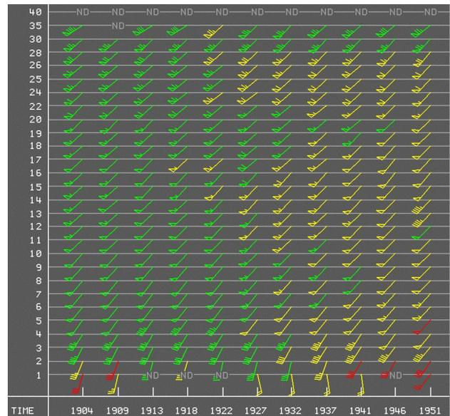
Figure 5. AKQ VWP from 1904 UTC to 1951 UTC with low level backing ahead of the storms at 1927 UTC and veering as the storms arrived at 1951 UTC.
