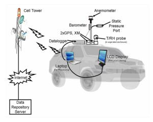
Figure 7: Overview of a basic MM vehicle implementing MRESS technology while in the field.
