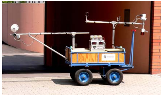
Fig. 4: Mobile human-biometeorological measuring system applied in the project KLIMES ALUF
