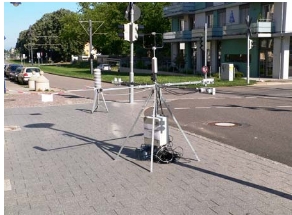
Fig. 22: Steady human-biometeorological measuring system at the NEE oriented sidewalk within a WNW-ESE oriented street canyon in Freiburg, Vauban, view to NW
