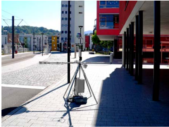
Fig. 23: Steady human-biometeorological measuring system at the NEE oriented sidewalk within a WNW-ESE oriented street canyon in Freiburg, Vauban, view to E
