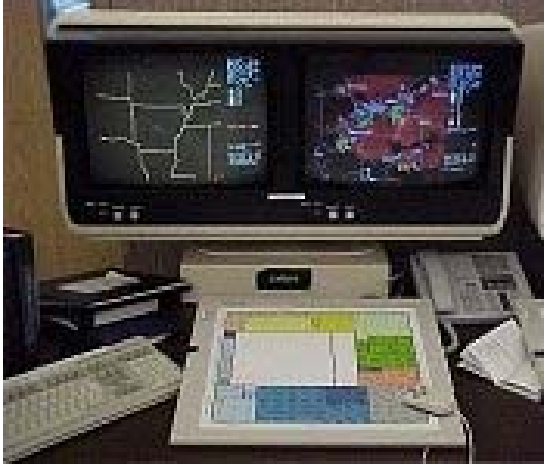
Figure 2. Principal User Processor. The 1980s predecessor to today's radar analysis in AWIPS.
