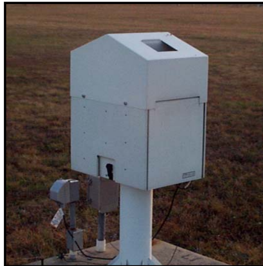
Figure 1. National Weather Service ceilometer model K220 (range 4000 meters)
