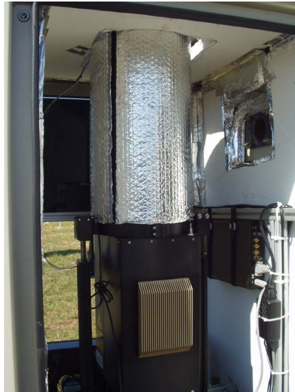
Figure 4. Micropulse Lidar inside conditioned housing
