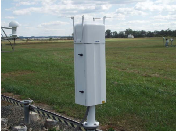
Figure 2. National Weather Service ceilometer model CL31 (range 8000 meters)
