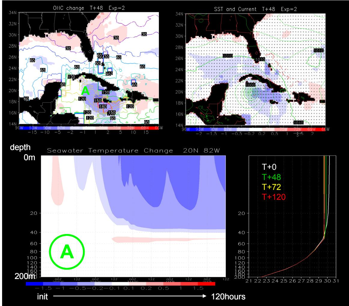
FIGURE 4. Impacts of coupling with the ocean model in the cyclone development stage. Upper left panel shows ocean heat content (contour, in  $\text{kJ}/\text{cm}^2$ ) and its change from initial time to 48hours integration (by shaded). Upper right panel shows SST change (in degree C) from initial time to 48hours integration as shaded. Lower panels show changes in seawater temperature up to 200m depth (in degree C) at the location “A” indicated in the upper left panel.
