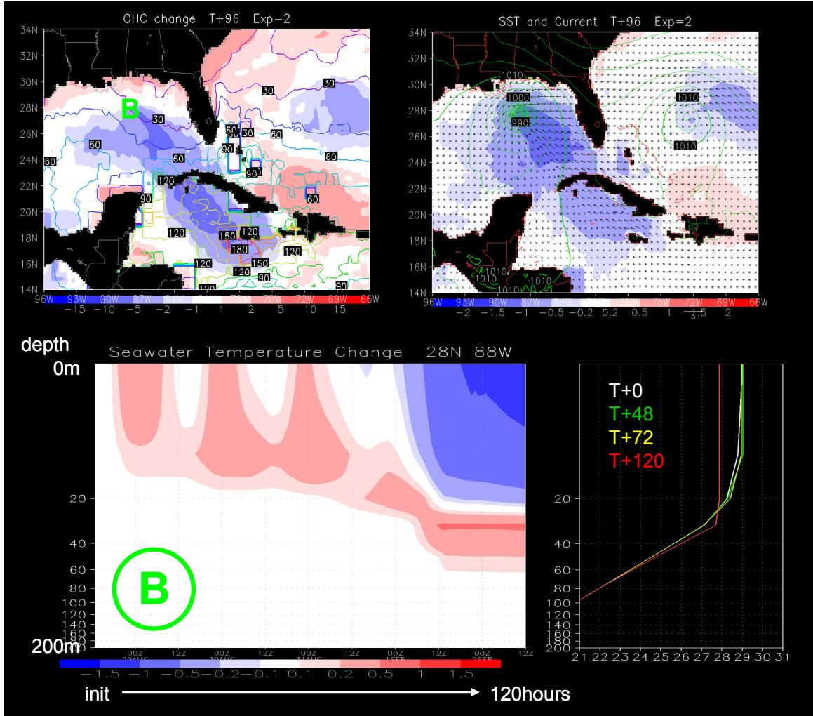
FIGURE 5. Same as figure 4, but for the cyclone weakening stage. Upper left shows OHC and its change up to 96hours integration, and upper right does SST change at 96hours later. Lower panels show changes in seawater temperature for the location “B”.
