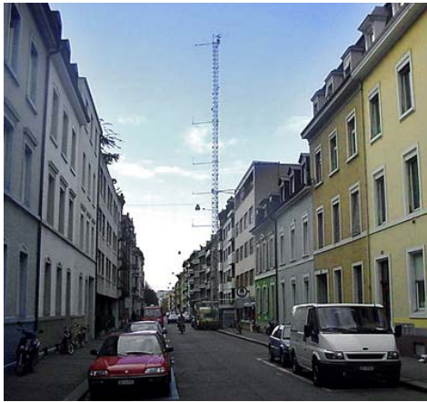
Figure 2. The left panel shows the meteorology mast in the BUBBLE experiment (Rotach et al., 2004) where measurements represent the roughness sub-layer. The right panel is from the Copenhagen experiment (Gryning and Lyck, 1984) where the measurements were performed above the roughness sub-layer.
