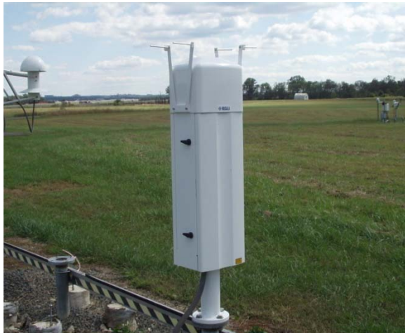
Figure 2. National Weather Service ceilometer model CL31 (range 8000 meters)
