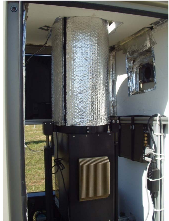
Figure 3. MicroPulse Lidar inside conditioned housing
