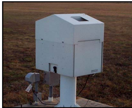
Figure 1. National Weather Service ceilometer model K220 (range 4000 meters)
