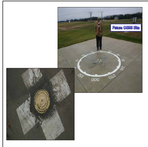
Figure 1. NGS Benchmark and future CORS site installed at the SFSC.
