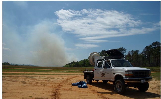
Figure 1: UMass W-band mobile radar and lidar system observing smoke plume at Fort Benning on April 11, 2008
