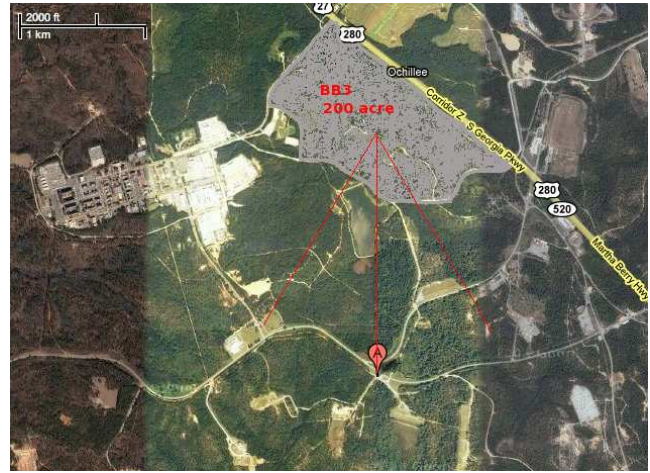
Figure 2: A map of the prescribed burn zone(shadowed) and instrument location on April 15, 2008. UMass W-band system is oriented north-south at marker A, about 1.6km from the center of burn zone.
