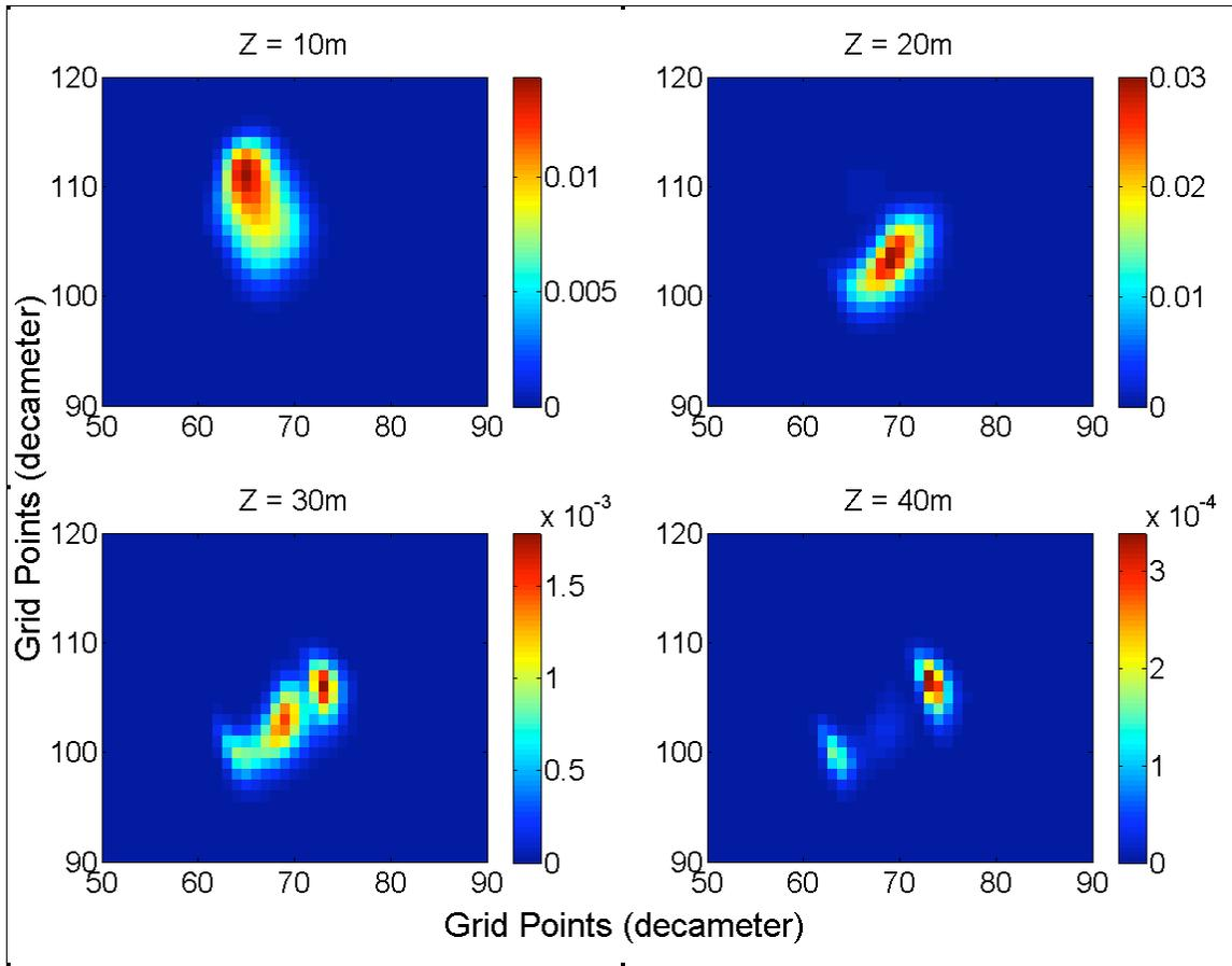
Figure 2. Concentration CFD data at 10, 20, 30 and 40 meter height levels at 40 seconds.
