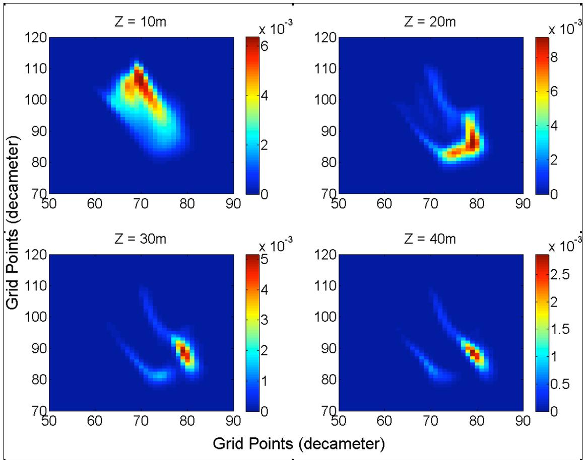
Figure 3. Concentration CFD data at 10, 20, 30 and 40 meter height levels at 90 seconds.
