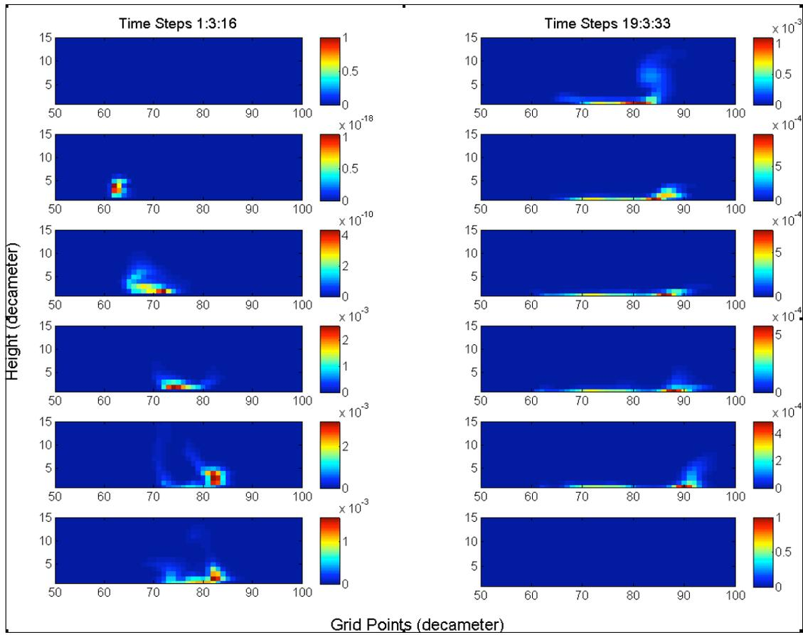
Figure 1. Along wind perspective of CFD concentration data at the 80<sup>th</sup> x direction grid point, for five minutes at 30 second intervals.
