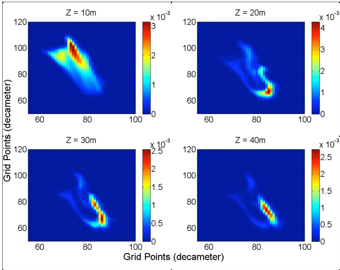
Figure 4. Concentration CFD data at 10, 20, 30 and 40 meter height levels at 140 seconds.
