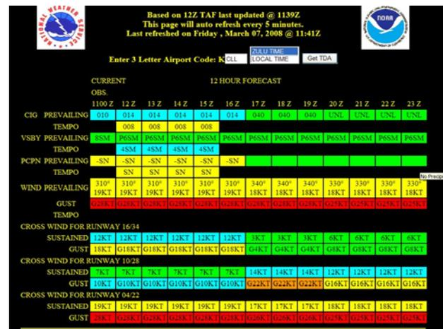
**Fig. 5** Example Decision Aid showing the different crosswind calculations for each runway at Easterwood Field, College Station, TX (KCLL).
