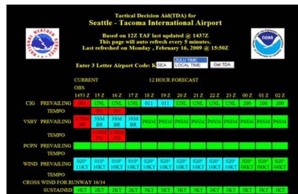
**Fig. 3** Example Decision Aid showing Low Instrument Flight Rule (LIFR) conditions occurring and temporarily forecast for Seattle-Tacoma International Airport (KSEA).
