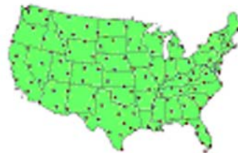
Figure 4.1 Current NLDN map. System is comprised of 114 lightning sensors locations across the continental US [Source: Vaisala, 2004.]
