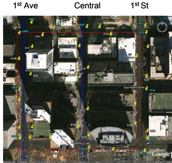
Figure 1: Sketch of the study area in downtown Phoenix adapted from Google Earth. The red line encompasses the area investigated using a hand-held IR camera. Yellow marks show measurement positions.
