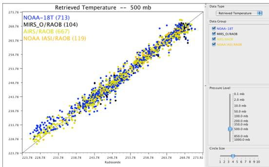
**Figure 6: Scatter plot with ground truth (radiosonde) plotted along X-axis and satellite temperature values plotted along Y-axis.**
