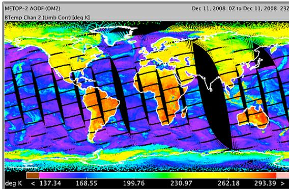
**Figure 7: EDGEIS image of AMSU-A brightness temperature data from the NOAA MetOp-2 satellite system.**
