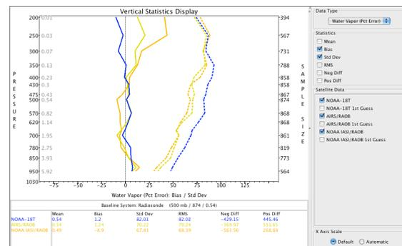
**Figure 5:** Vertical accuracy graph showing bias (solid line) and standard deviation (dashed line) for NOAA-18, AIRS and NOAA IASI.
