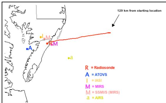
**Figure 4:** Example of individual set of collocated radiosonde (red) and respective satellite observations (other colors) and the associated drift (red line) of the radiosonde during flight in vicinity of Ocean City, Maryland on January 2, 2009.
