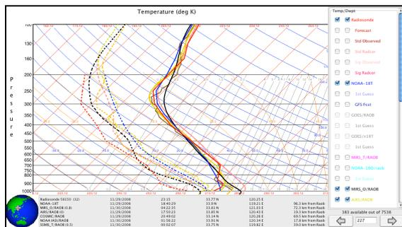
**Figure 2:** The main graph window in PDISP showing temperature (solid lines) and moisture (dashed lines) profiles from several satellite systems.
