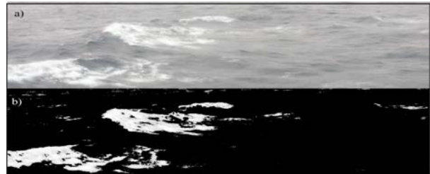
Figure 1 a) Digital image of the sea surface obtained from the bridge-mounted camera on Discovery (taken on March 30 2007), and (b) the same image with a mask derived from AWE image processing (Callaghan and White, 2008) applied to isolate the whitecaps.
