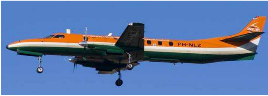
Figure 7 NLR's Swearingen Metro II aircraft, a twin turboprop modified for aerospace research. (Image provided by NLR.)
