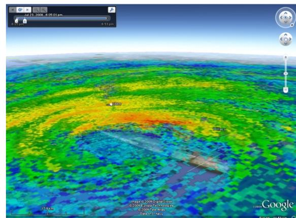
**Figure 12** – View of Hurricane Dolly's eyewall from 1800 to 1805 UTC on 23 June 2008, looking from the NE. Four NEXRAD elevations are shown for r0 (0.5°), r1 (1.45°), r2 (2.40°) and r3 (3.35°). A sample kmz is available online for demonstration of 4D animation over the hour using Google Earth.
