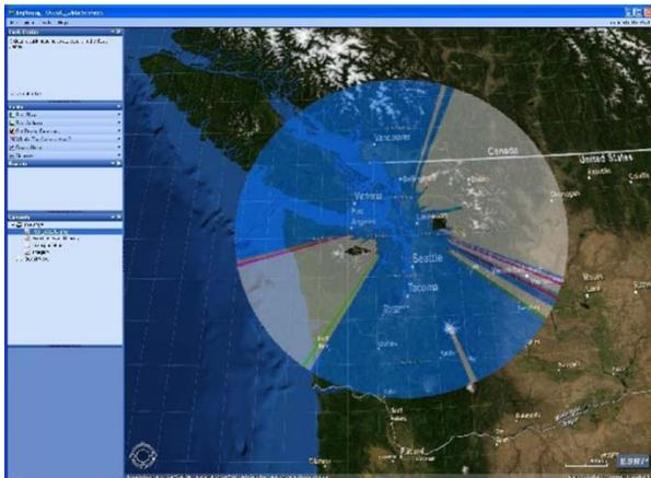
**Figure 8** – Occultation pattern for the lowest elevation scan of Seattle, WA NEXRAD (station KATX) in ArcGIS Explorer. The occultation pattern is a 3D service draped upon beam centroid elevation. Virtual Globe features are similar to Google Earth as shown in Figure 7.
