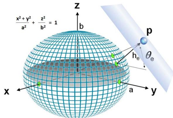
**Figure 5** – Google Earth COLLADA models are drawn on the tangent plane. GE claims to adopt the WGS-84 spheroid.
