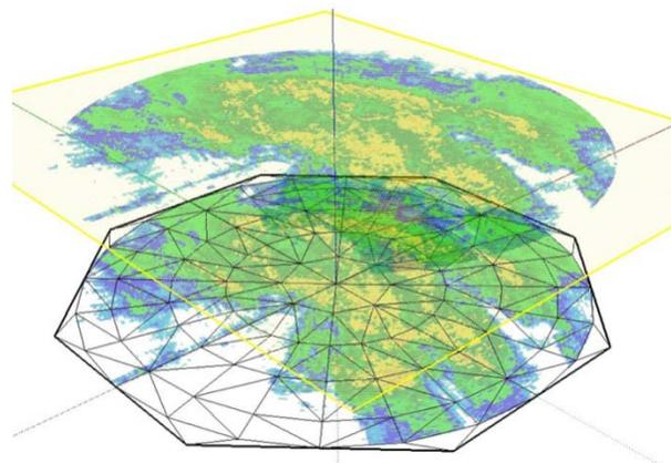
**Figure 6** – Google Sketchup drawing of the radar beam propagation surface for 0.5 degree elevation, defined w.r.t. the tangent plane. Radar polar plot images are draped onto this surface.
