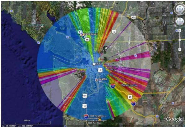
**Figure 7** – Occultation pattern for the lowest elevation scan of Seattle, WA NEXRAD (station KATX) in Google Earth. Note total blockage of this elevation scan by terrain to the East and West, and by Mt. Rainier to the SSE. Areas where the terrain layer is higher than the beam centroid can be seen penetrating the coverage.
