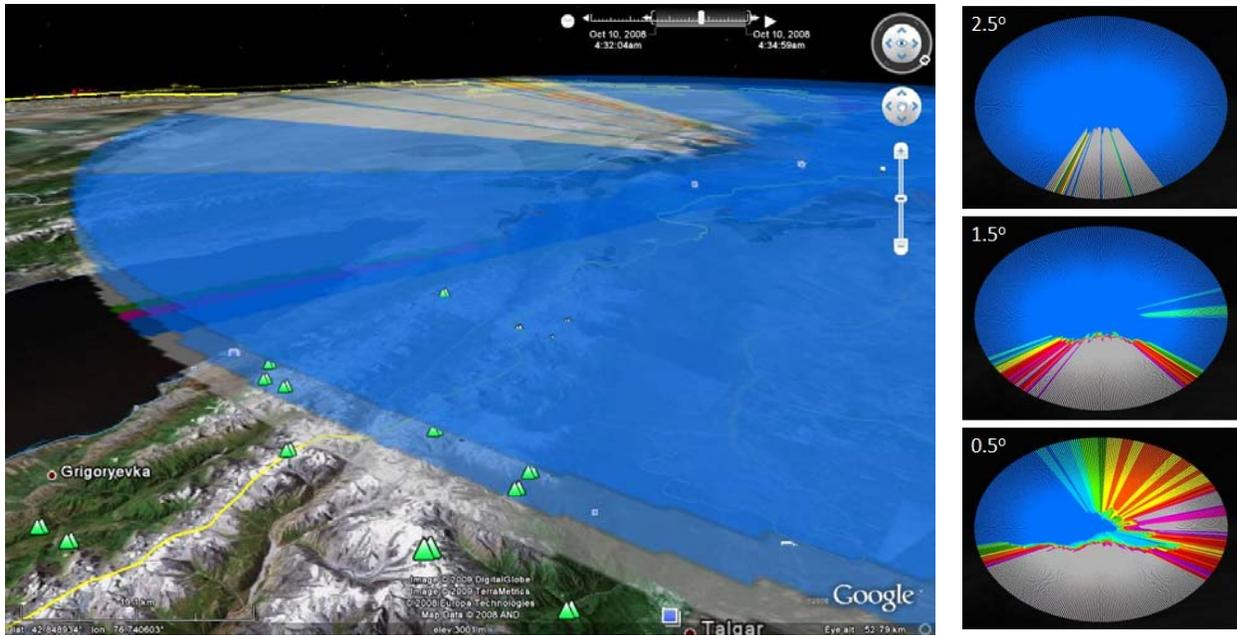
**Figure 10** – Occultation for a hypothetical weather radar system at Manas International Airport, Bishkek, Kyrgyzstan. PPI occultation patterns for three primary elevations [0.5, 1.5 and 2.5 degrees] are inset to the right.
