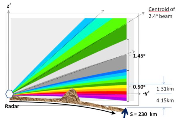
**Figure 2** – Adapted from FMH-11 (2005) for Virtual Globe geometry with WGS-84 horizontal datum. When Earth curvature is included, radar beam propagation paths can be seen to refract downwards “towards” the Earth surface.
