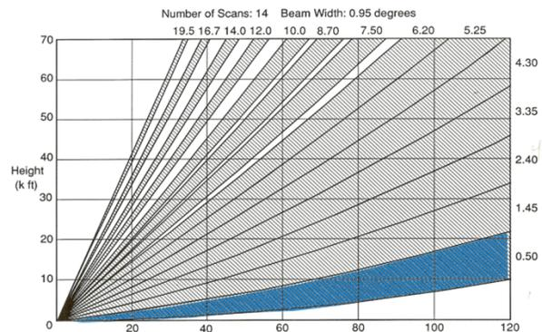
**Figure 1** – Flat Earth geometry, from FMH-11 (2005). Although radar beams are normally refracted downward “towards” the Earth surface, flat Earth plots add Earth curvature, so they appear to go “up”. Compare with Figure 2.
