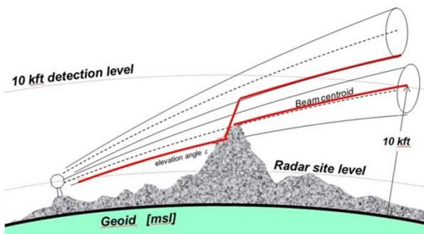
**Figure 9** – Radar propagation paths, showing occultation of the lowest elevation beam by terrain. If more than 50% of a beam is removed by occultation, then that beam is considered blocked and radar signals are obtained from the next higher elevation scan.
