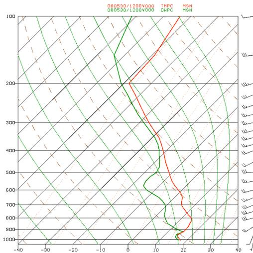
Figure 11 Initial sounding for the WRF model over Madison Wisconsin from the 12 UTC NAM model grids.
