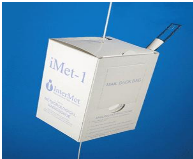
Figure 1. The iMet-3000 403 MHz ground station (top), and the iMet-1 radiosonde (bottom), for more information see http://www.intermetsystems.com .
