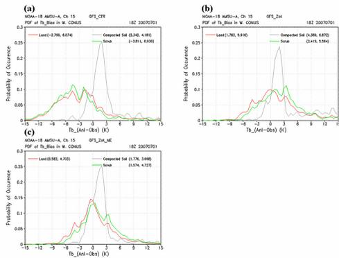
Fig.4. PDF of Tb bias for all clear sky pixels within the western CONUS (red box in Fig. 3) from the control run (a), new roughness sensitivity run (b), and new emissivity with new roughness run (c). Tb biases (first in parentheses) and rmse (second in parentheses) for various land surface category are also given.
