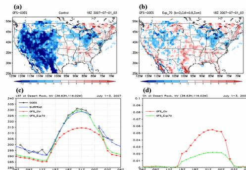
Fig.1. Comparison of land skin temperatures simulated in GFS and verification with the observations. (a) difference between GFS and GOES in the control run at 1800 UTC; (b) difference between GFS and GOES in the sensitivity run at 1800 UTC; (c) verification of diurnal change with GOES (black) and SURFRAD (blue) at Desert Rock, NV; red and green lines are for control run and sensitivity runs, separately;(d) diurnal change of aerodynamic conductance at Desert Rock.
