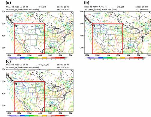
Fig.3. Horizontal distribution of satellite pixels used in GSI: brightness temperature bias of Channel 15, NOAA-18 AMSU-A from control run (a), new roughness sensitivity run (b), and new emissivity with new roughness run (c).
