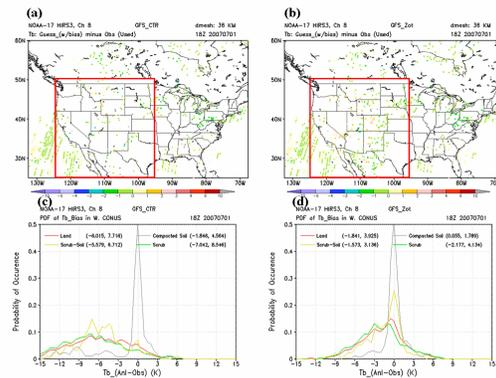
Fig.2. Horizontal distribution of satellite pixels used in GSI: brightness temperature bias of Channel 8, NOAA-17 HIRS3 from control run (a) and sensitivity run (b). PDF of Tb bias for all clear sky pixels within the western CONUS (red box) from the control run (c) and the sensitivity run (d). Tb biases (first values in parentheses) and rmse (second values in parentheses) for various land surface categories are also given.
