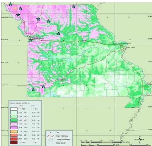
Figure 1. The green stars represent the location of each tall tower location overlaid on the AWS Truewind map of projected wind speeds at 100 m.
