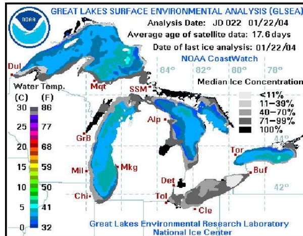
Figure 2.2 Gridded lake temperature and ice coverage for the Great Lakes. From the Great Lakes Environmental Research Laboratory.
