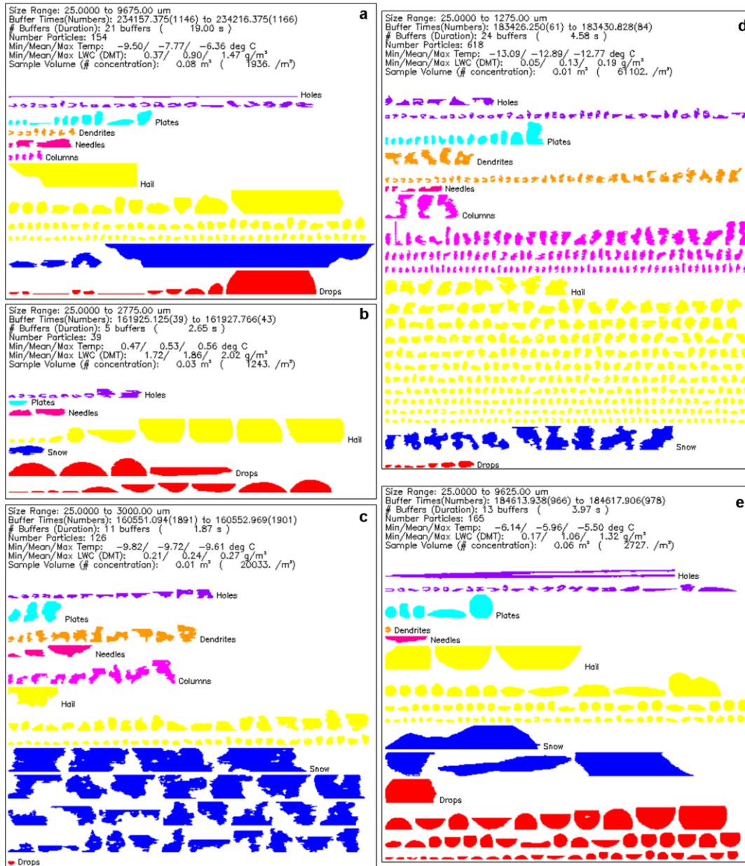
Fig. 1. Example particle images from the 2D-C probe with classifications given by Feind (2006). Note that each image set includes a variety of particle types. Final classifications used in this study are exemplified by a) hail, b) drops c) snow, d) graupel, and e) drops/graupel.
