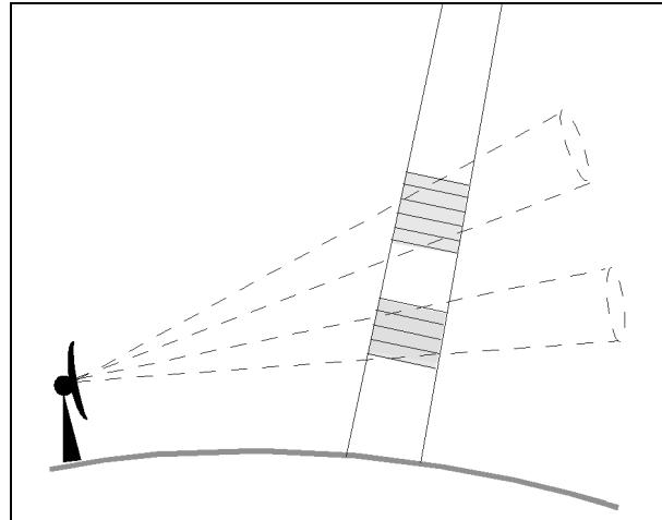
**Figure 1.** Schematic of PR gate averaging at GR sweep intersections. Shaded areas are PR gates intersecting two GR sweeps (dashed) at different elevation angles. Only one PR ray is shown. PR gates are 250 m along-ray by ~5 km in the horizontal.
