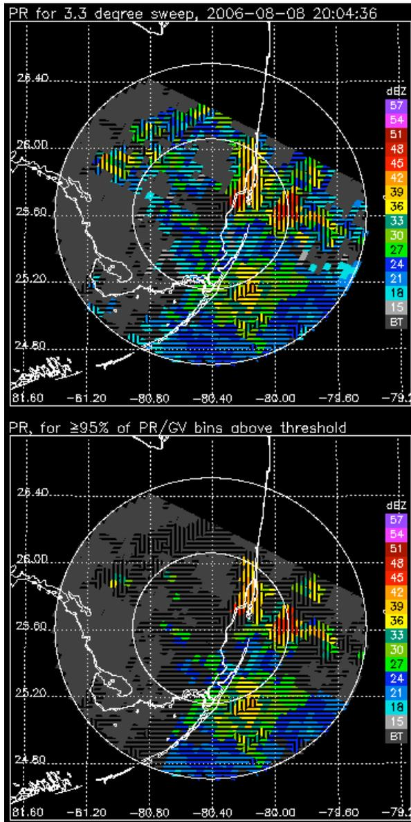
Figure 4. Total (top) and filtered (bottom) PR volume-matched data for the case in Fig. 3, but at 3.3° elevation. Data where 5% or more of the PR or GR gates in the volume averages were below reflectivity thresholds are grayed-out in the lower PPI.
