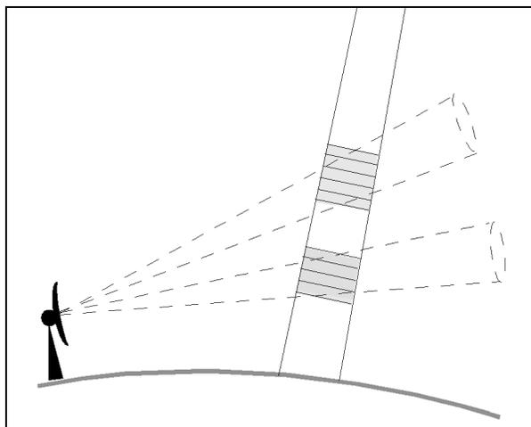
**Figure 1.** Schematic of PR gate averaging at GR sweep intersections. Shaded areas are PR gates intersecting two GR sweeps (dashed) at different elevation angles. Only one PR ray is shown. PR gates are 250 m along-ray by ~5 km in the horizontal.
