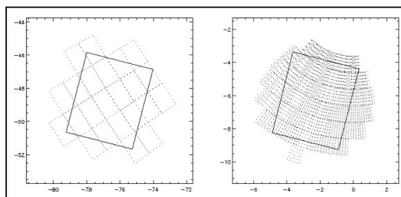
**Figure 2.** Schematic of ground radar bins (dotted) horizontally averaged over a near-circular area centered on a PR footprint (solid) plotted as a rectangular area, at far (left) and near (right) ranges from the GR. Axes show x- and y-distance from GR, in km.
