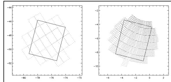
**Figure 2.** Schematic of ground radar bins (dotted) horizontally averaged over a near-circular area centered on a PR footprint (solid) plotted as a rectangular area, at far (left) and near (right) ranges from the GR. Axes show x- and y-distance from GR, in km.
