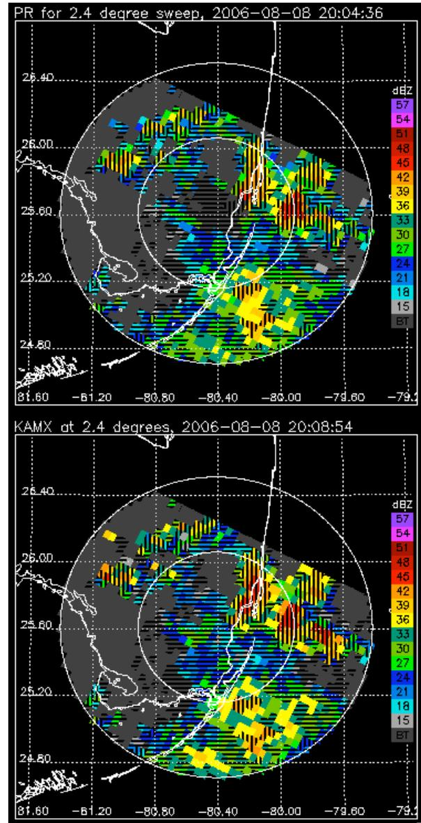
**Figure 3.** PR (top) and GR (bottom) volume-matched data for the KAMX (Miami, FL) PR overpass at 2004 UTC on 8 August 2006, on the 2.4° elevation sweep, plotted as PPIs. Vertical (horizontal) [no] hatching indicates convective (stratiform) [unknown] rain type.
