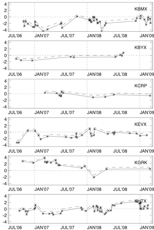
**Figure 5.** Time series of PR-GR mean reflectivity difference (dBZ) for stratiform precipitation above the melting layer, for six WSR-88D sites in the VN. Solid (dashed) lines plot differences using original (frequency adjusted) GR data.
