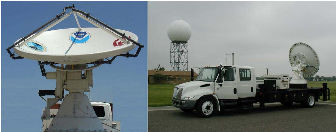
Fig. 1. XERES mobile radar: (left) the antenna, (right) the radar deployed near the WSR-88D KOUN for the experiment.
