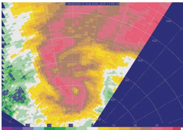
Fig. 4. Unedited radar reflectivity (dBZ) from the MWR-05XP at  $2.5^\circ$  elevation angle, of the parent supercell for the tornado seen in Fig. 3. Range markings shown every 2 km. Tornado was located at the weak-echo hole seen at 5.5 km range.
