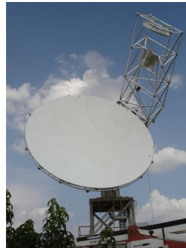
Fig. 16: Antenna in 135^\circ position on the test range.
