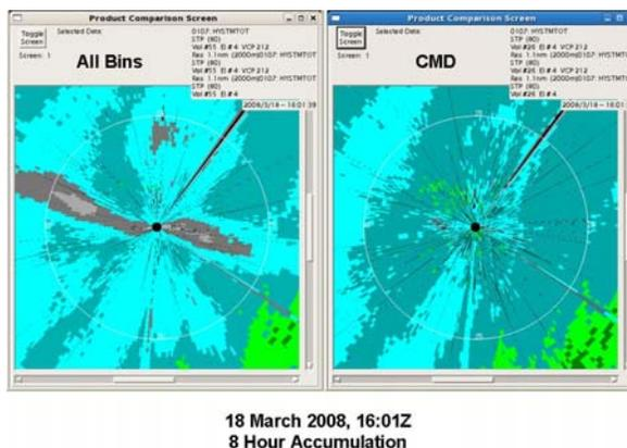
**Figure 15 - Precipitation Accumulation Near the Radar, All Bins vs. CMD Control**
