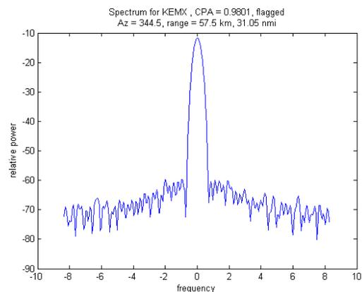
**Figure 18 - Spectrum of a Normal Clutter Target**
