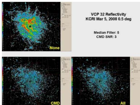
**Figure 4 - Clear Air Ground Clutter Identification Test, Reflectivity March 5, 2008, KCRI**
