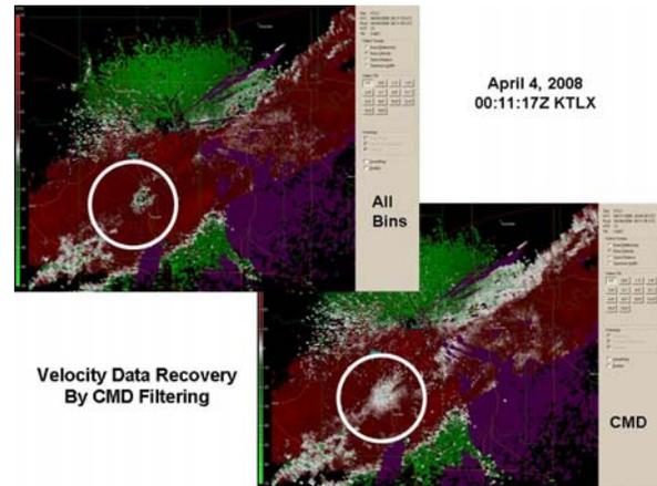
**Figure 9 - Velocity Images, April 4, 2008, All Bins vs. CMD Control**
