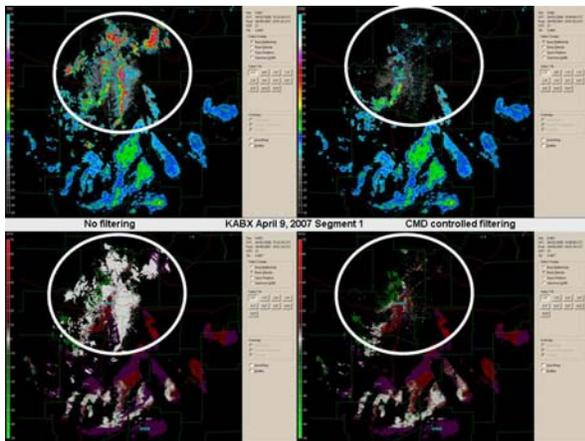
**Figure 11 - Albuquerque NM Clutter Removed by Dynamic CMD Control**
