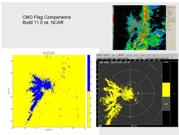
**Figure 12 - NCAR and Build 11.0 CMD Flag Generation Comparison**
