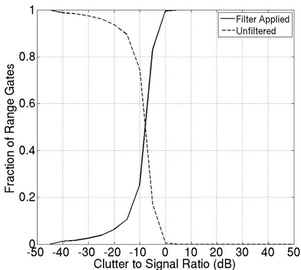
**Figure 2 - CMD Clutter Detection, Single Polarization Case (Courtesy John Hubbert, NCAR)**
