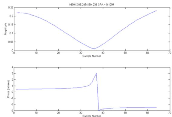
**Figure 21 - Magnitude and Phase Plots, Low Coherency Clutter Target**
