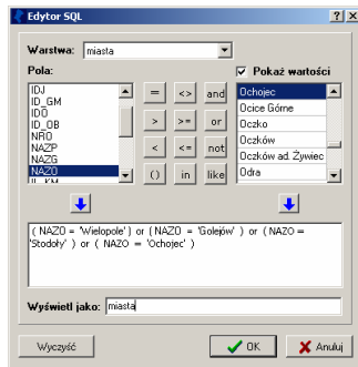
Fig. 17. Window with simple SQL query: creation of a new GIS layer for the selected object.
