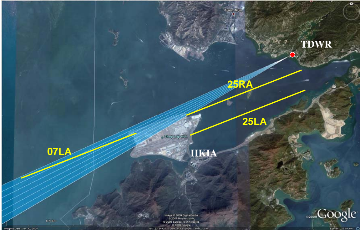
Fig.1 The locations of the Hong Kong TDWR (red dot) radar and Hong Kong International Airport (HKIA). The blue beams illustrate the radar beams over the runways corridor 07LA of the airport with 1° azimuth interval. Three yellow lines indicate the approach paths and their names are marked.
