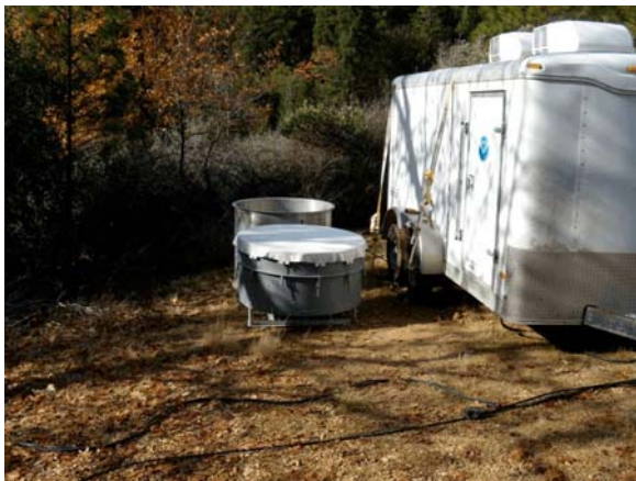
Figure 2. Prototype FM-CW radar installed at the Colfax, CA HMT field site in December 2008.
