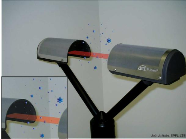
Figure 2: The optical disdrometer Parsivel (OTT) providing DSD measurements based on the attenuation of the laser signal when a particle crosses the beam.
