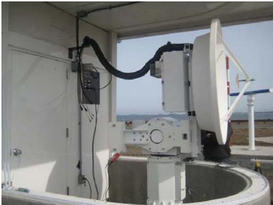
Fig. 3. W-Band Radar Antenna and Pedestal.
