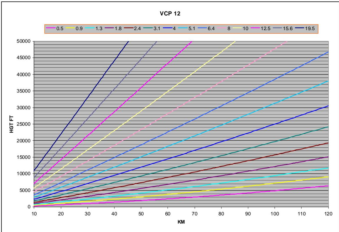
**Figure 4: VCP 12 Elevations Plotted on Range / Height Grid**
