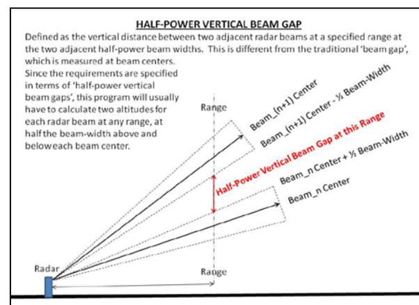
Figure 1. Depiction of the half-power beam gap. The half-power vertical beam gap is defined as the vertical distance between two adjacent radar beams from the bottom of the upper half-power beam width to the top of the lower half-power beam width, as shown above. The half-power beam width of the new radar is 0.95°.
