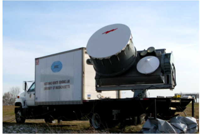
Figure 8: AMFR : The large antenna at left is for Ku-band, at the lower right is Ka-band and two W-band antennas at the upper part of the platform, can be pointed in both azimuth and elevation.
