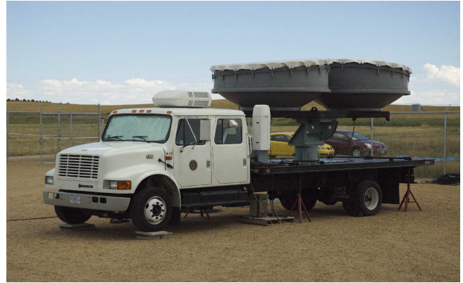
Figure 6: S-band FMCW radar deployed at Boulder Atmospheric Observatory, Aug 2007.
