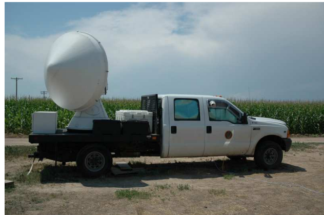
Figure 3: The X-Pol mobile radar deployed for refractivity measurements in Colorado, July 2005.
