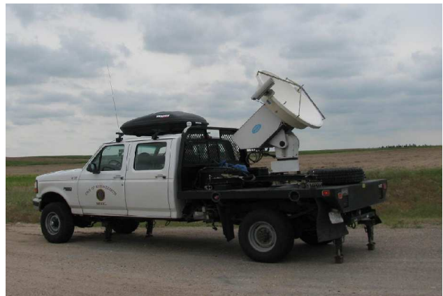
Figure 1: W-band radar performing a clear-air VAD scan during Vortex2.
