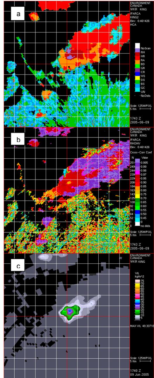
Figure 6. (a) iParCA classification output for storm cell at 1740 UTC 2005-Jun-09. (b)  $\rho_{HV}$  (c) VIL. Red crosshairs is at 47 km  $339^\circ$  from the radar.
