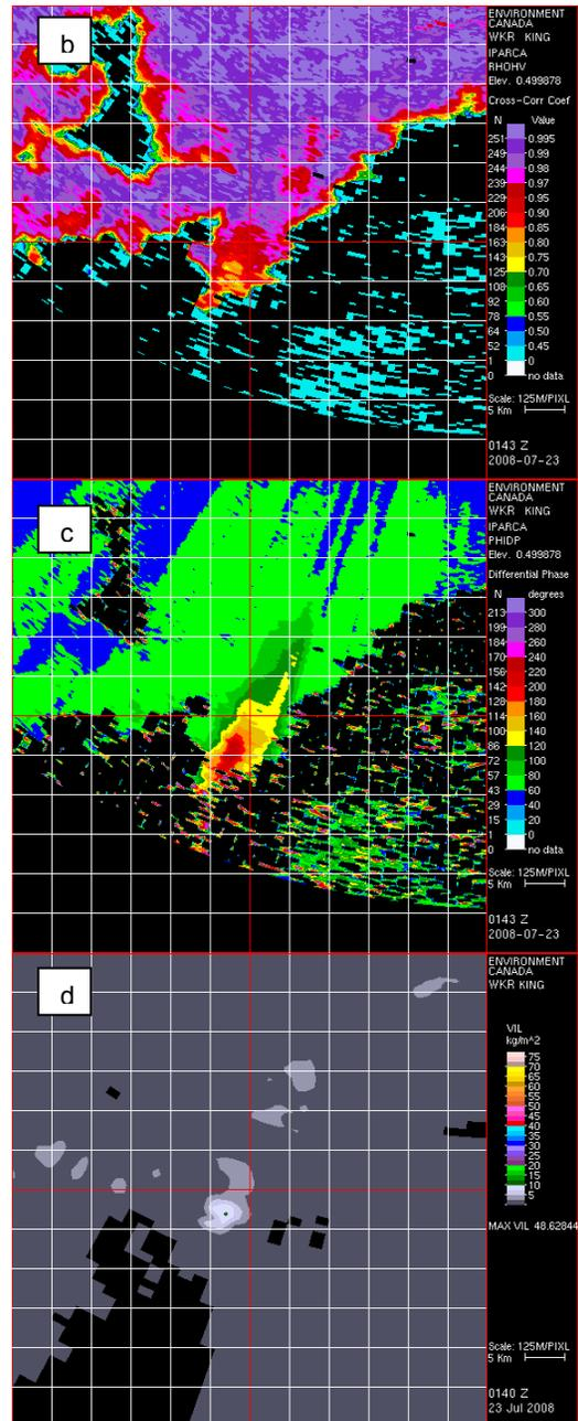
Figure 4. (a) Corrected horizontal reflectivity ( $Z_{corr}$ ), (b)  $\rho_{HV}$ , (c)  $\Phi_{DP}$  and (d) VIL at 0140 UTC on 2008-Jul-23. Red cross hairs are at 94 km and  $201^\circ$  from the radar.
