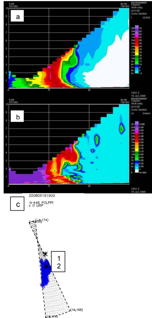
Figure 3. Vertical cross-section of Z<sub>H</sub> (a) and ρ<sub>HV</sub> (b) for a storm cell close to the radar at 1900 UTC 2008-Jun-16. (c) iParCA hail pixels (blue) locations from the 0.5° POLPPI scan. Asterisks 1 and 2 marks specific pixel locations referred to in the text.
