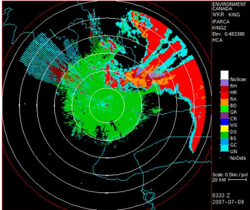
Figure 2. Example output from the iParCA algorithm at 0300 UTC 2007-Jul-21 from the high resolution 0.5° POLPPI scan. Range rings are 20 km apart.
