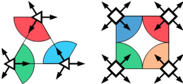
Figure 4: Competing topologies for a deployment of polarimetric PAR; triangular topology with 3 PAR panels per radar site (left) and square topology with 4 PAR panels per radar site (right).
