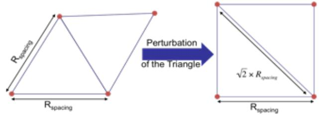
Figure 5: Square topology as a perturbation of the equilateral triangle topology.
