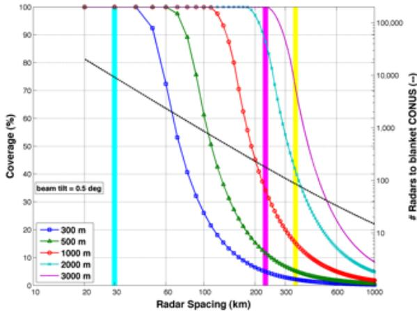
Figure 6: Coverage and number of radars plot for square topology.
