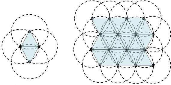
Figure 2: Network topology for a CASA-type dense radar network: radars with 40 km range placed 30 km apart to form a mesh of equilateral triangles. The network of the left is the basic topology of the CASA IP1 testbed network deployed in southwestern Oklahoma. The network on the right shows a larger four row, four column example.
