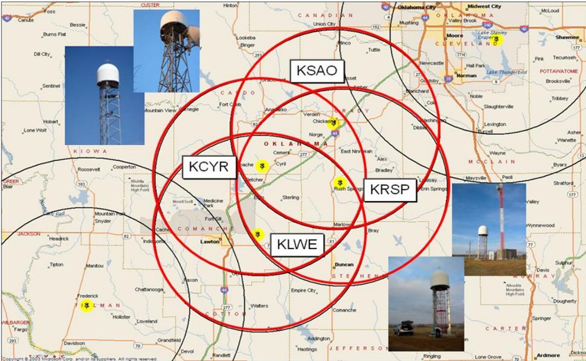
Fig. 1: The four CASA radar sites are located near the cities of Cyril (KCYR), Lawton (KLWE), Rush Springs (KRSP), and Chickasha (KSAO). Range rings of 40 km are shown in red around each CASA radar. The nearest NEXRAD radars are KTLX and KFDR; range rings of 40 km and 60 km are shown.
