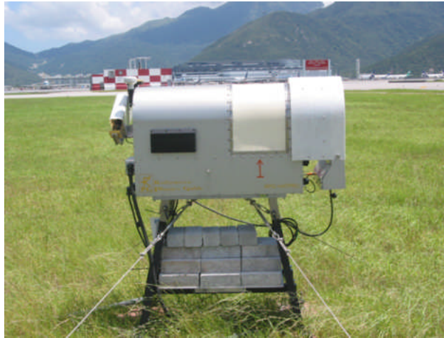
(a) The microwave radiometer at the Hong Kong International Airport
