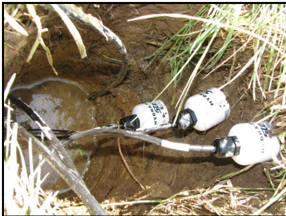
Figure 5. Sensors installed at 5, 10, and 20 cm.
