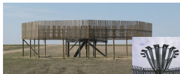
Figure 1: Schematic (top) and photo (bottom) of the Double Fence Intercomparison Reference or DFIR (Goodison et al 1998). A manually observed Tretyakov gauge (inset bottom right) is located in the centre of the fence structure.
