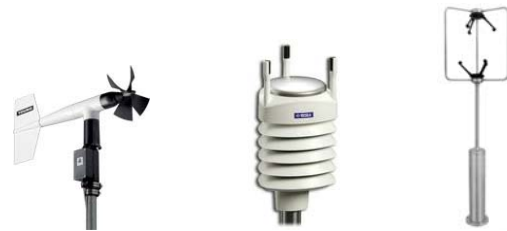
Figure 3. IMET R.M Young Propeller-Vane Vaisala WXT 520, and Gill WindMaster Pro Sonic Anemometer
