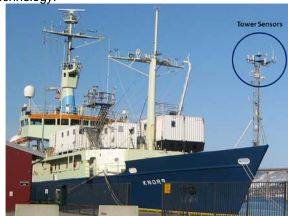
Figure 1. Tower sensors located on the forward mast on the bow of the Knorr.
