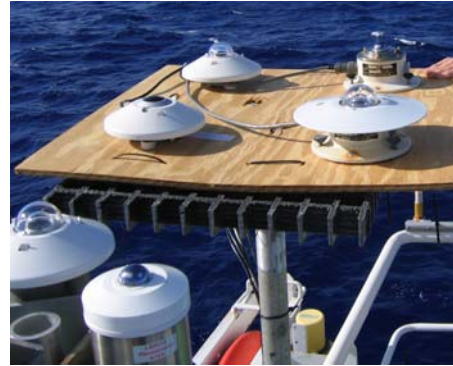
Figure 10. FLUX and WHOI standard radiometers setup for comparison.
