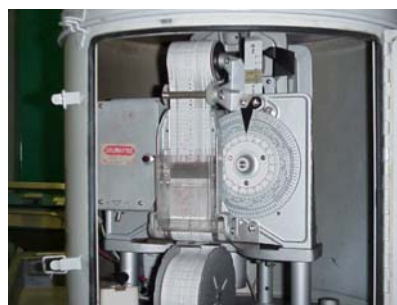
Figure 1. The inside of a Fischer & Porter gauge using punched-paper tape.
