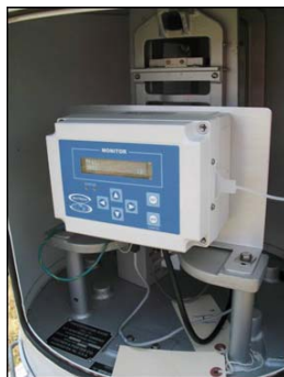
Figure 6. An example of a new precipitation recorder, which will replace the paper-tape assembly in Fischer & Porter rain gauges (U.S. Department of Commerce 2009).
