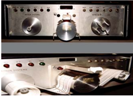
Figure 2. A MITRON reader evaluating punched-paper tape.
