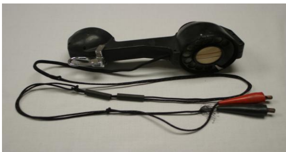
Fig. 6: Electronic communication handset with telephone rotary dialer.
